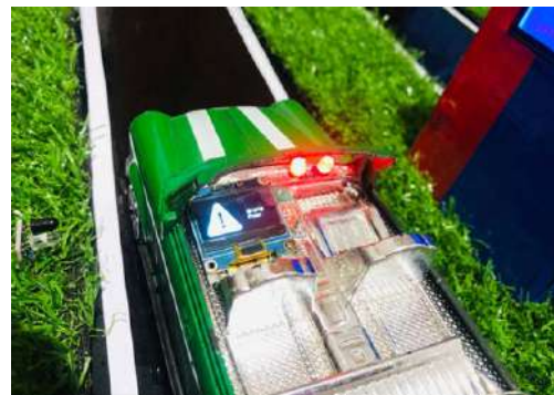
Figure 3: Alerting the driver due to oncoming road signal
